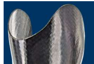
Composite on outside of lay-up
